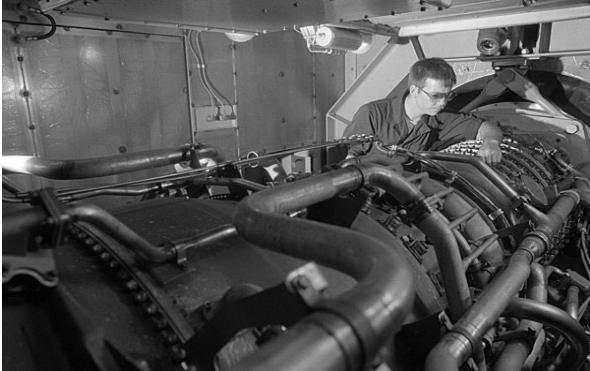
LM2500 Marine Gas Turbine Predominant turbine used in the U.S. Navy and 29 other navies
