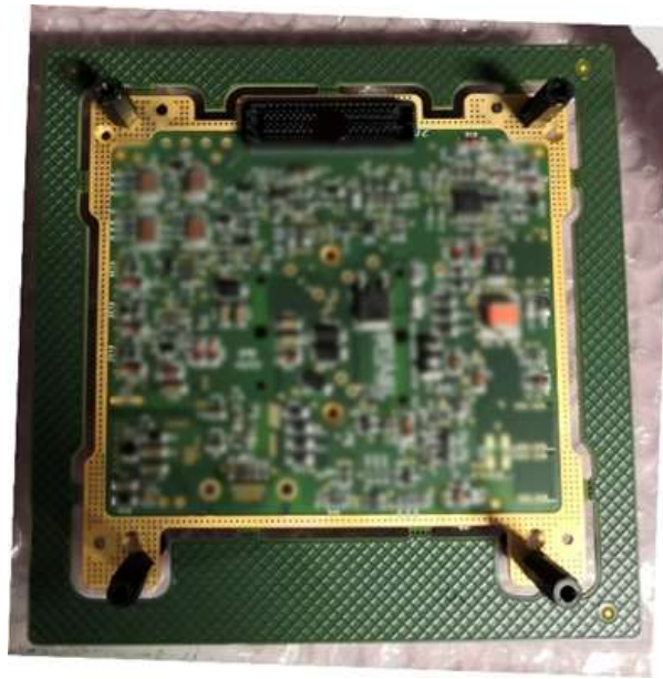
Figure 10: HPA_PCU Board
