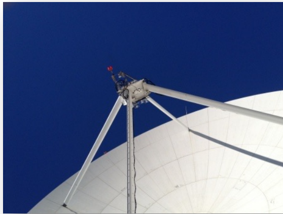
X-band Feed is located at the prime focus
