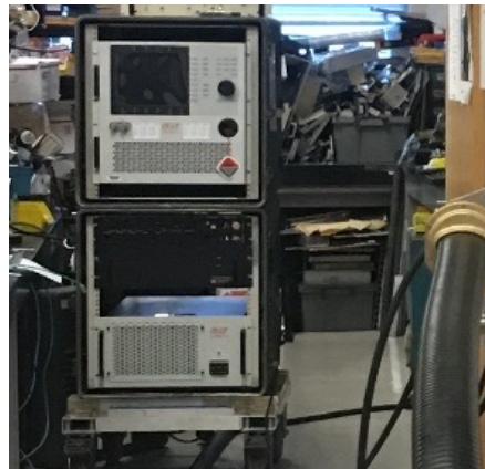
3 kW High Power Amplifier under test
