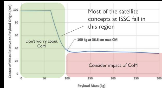
No more than 36 cm if total delivered payload is over 100 kg. Under 100 kg, CoM location is less critical.
