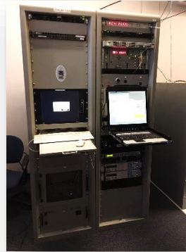
"Lite" Version of DSN Block 6 Exciter System Developed for Morehead State
