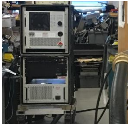
3 kW High Power Amplifier under test
