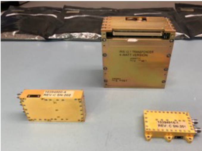
BioSentinel Iris Flight Unit including SSPA & LNA
