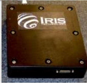
COTS AFRL developed AIM SX030 microcryocooler with cold finger to maintain detector at \leq 115K and iris controller
