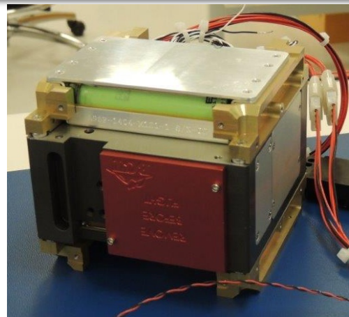
XACT ADCS unit sandwiched between 2 battery packs (top & bottom)
