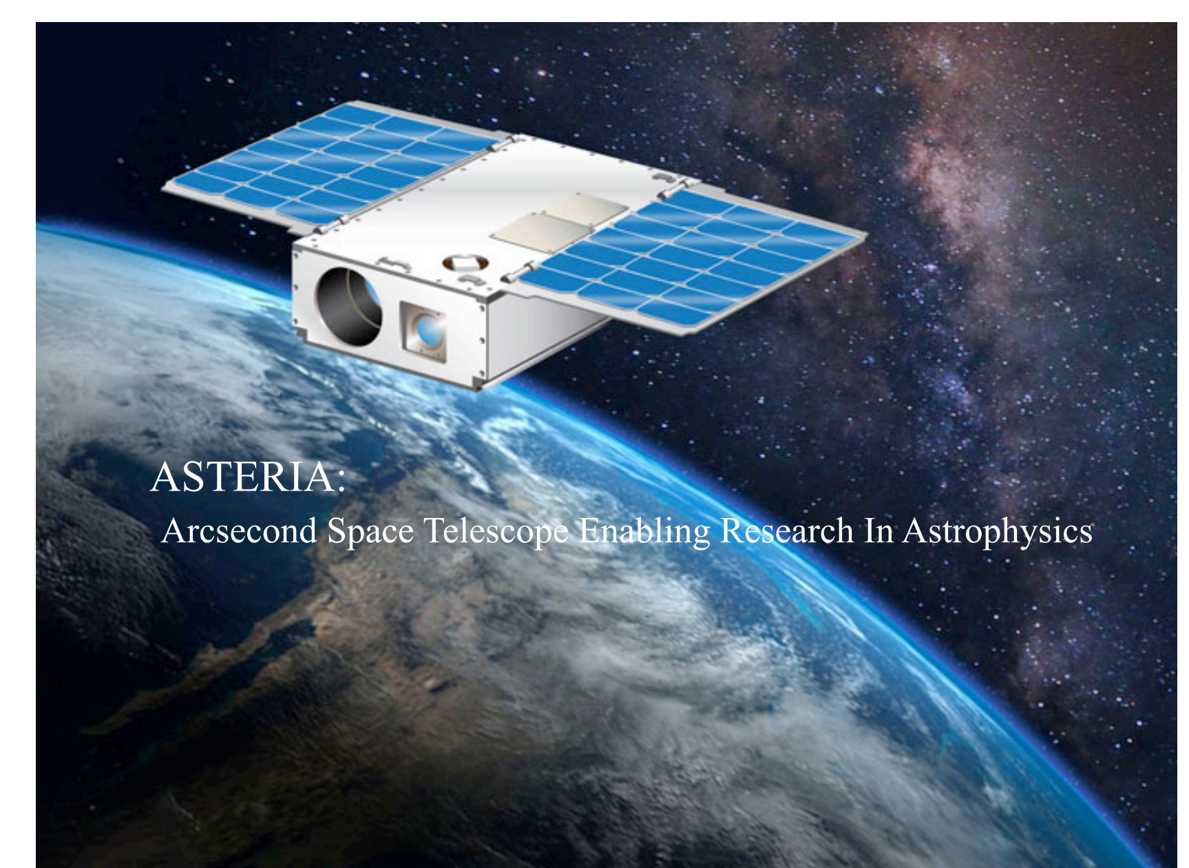
1 x 6U demo for two-stage pointing system to support exoplanet transit photometry
