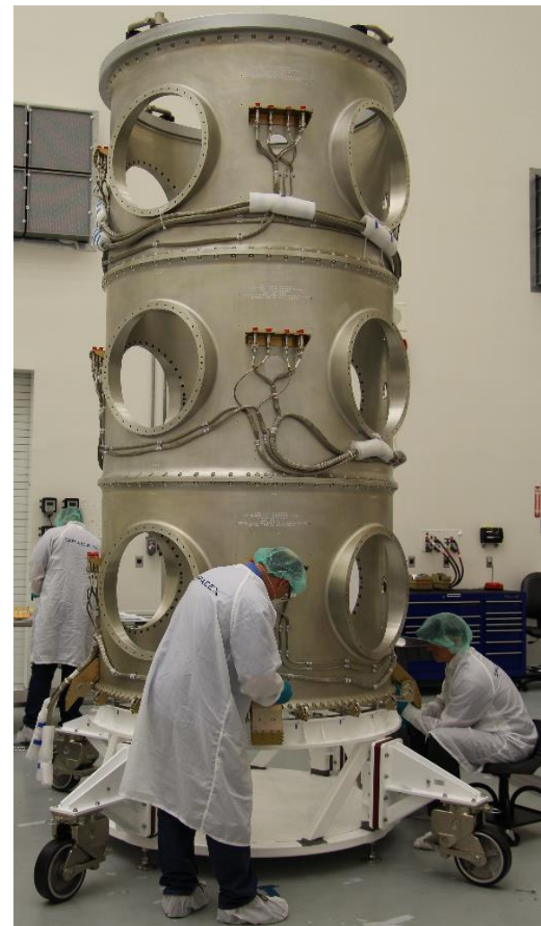
Moog engineers assembling dispenser stack (Photo Credit: ORBCOMM)
