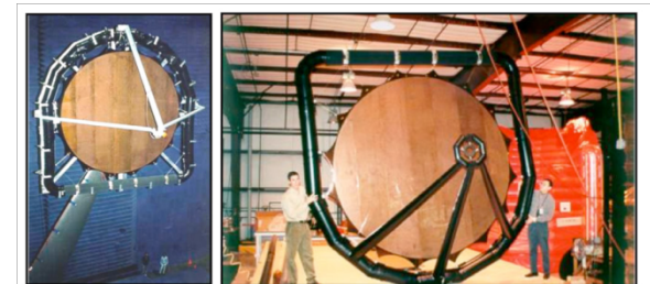
3m Ka-Band Inflatable Reflectarray Antenna (RF Test and Inflation Test)
