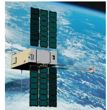
eHAWK MMA Solar Arrays (130 W/kg)
