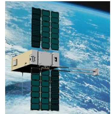
eHAWK MMA Solar Arrays (130 W/kg)
