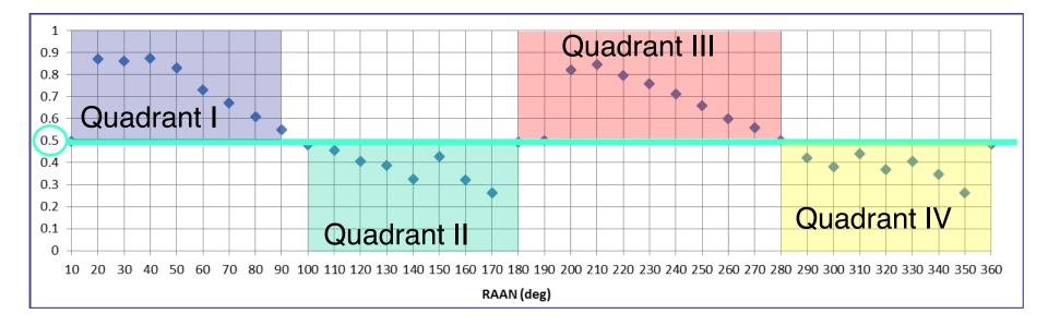
Earth escape trajectories can be thought of as being broken into 4 RAAN quadrants
