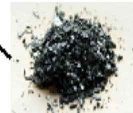
Iodine Propellant Stored as Solid Crystals; 300mTorr Storage Pressure
