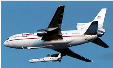
Air-launched space access, this from the launch of Space Technology 5
