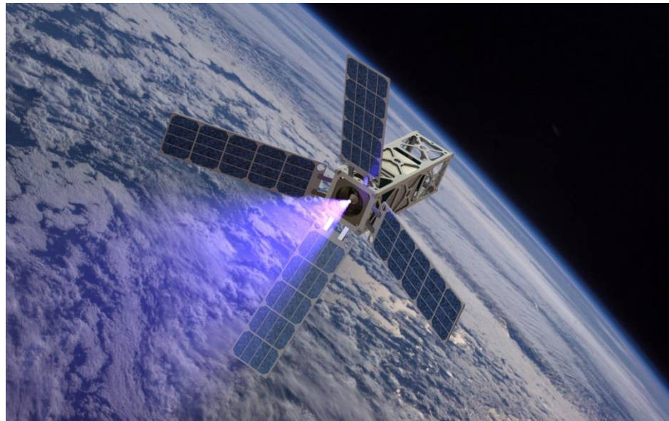
Design of a 3U 3U CubeSat with CAT engine performing initial testing in Low Earth Orbit.
