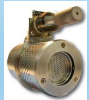
3 cm Micro RF Ion Thruster
